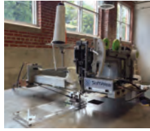
Softwear Automation’s ‘Sewbots’ improve production efficiency with a patented computer vision system. The machines use a combination of cameras and needles to track the placement of a fabric before sewing the apparel at a reported higher level of accuracy than the human eye.
