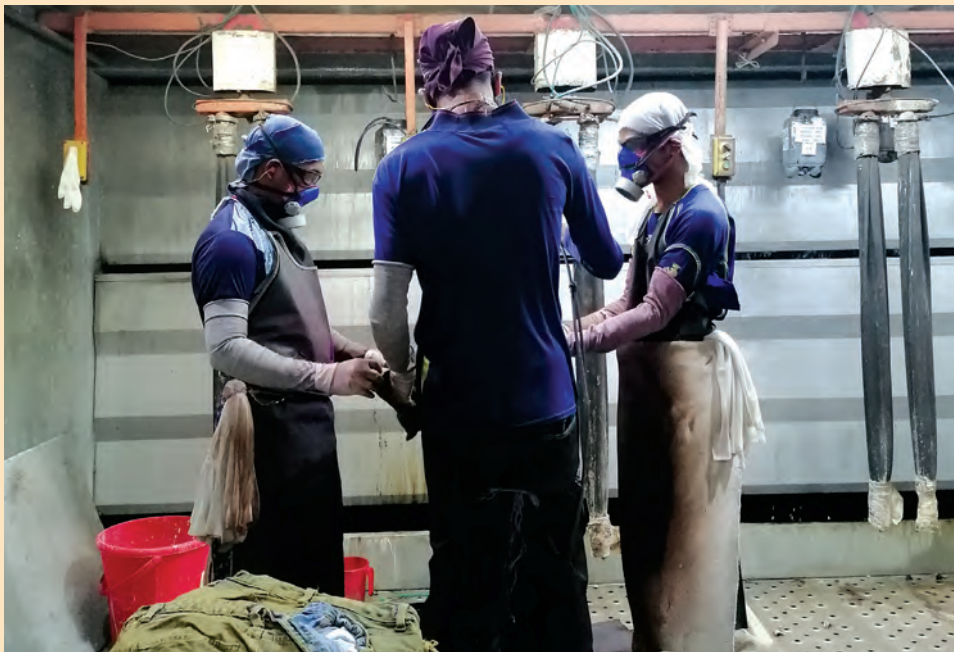
▼ Workers applying potassium permanganate to finish denim at a Tarasima Apparels denim mill, Dhaka, Bangladesh.
